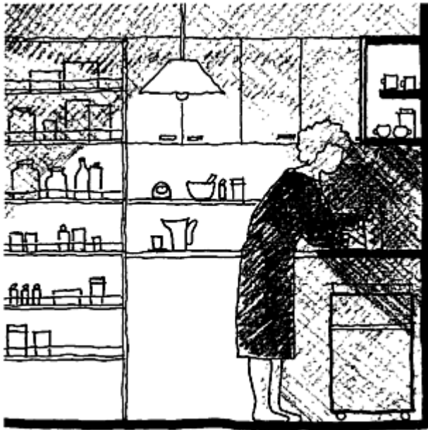
Fig. 5.4.4a: No task lighting, difficult to see
