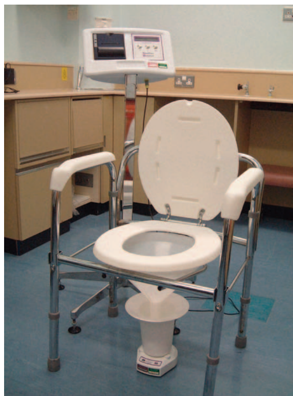
Figure 9.2 Portable urine flow meter used in a continence clinic.
